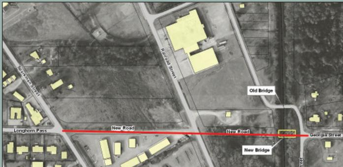
In early 2009, Longhorn Pass will be extended 1,500 feet across Railroad Street up to the new CSX bridge, 200 feet south of the old Hammitt Street Bridge. The new bridge will tie into Georgia Street on the east side of the tracks.
